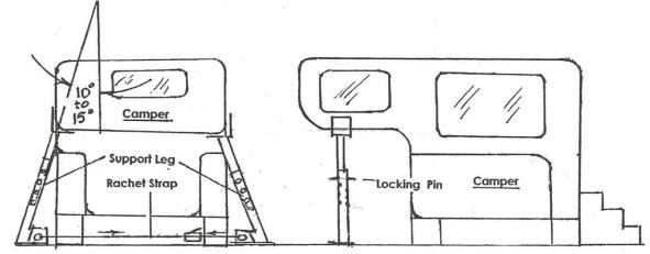
4. In performing step 3, thread the strap up through the slotted ratchet drum and pull the strap to get the slack out; then ratchet the strap until the support legs are snug and firmly supporting the overhang. Do not over- tighten the ratchet, as that could cause damage to the camper.
